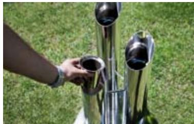
Place the burner(s) in the insert/ opening.
